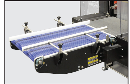
Optional pacing conveyor decelerates product as it enters the infeed conveyor
