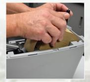
Remove cover to insert tape, then feed tape through slot.
