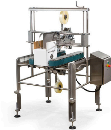
TBS-100 SA SEMI-AUTOMATIC Sanitary Top & Bottom Case Sealer w/ leg extensions
