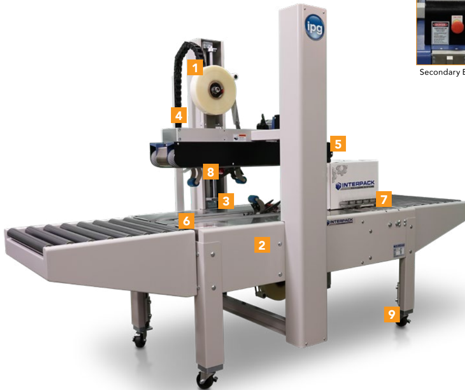
1 Tip-up tape head simplifies roll replacement
