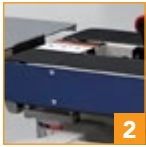
2 Bottom belt drive processes heavier cases
