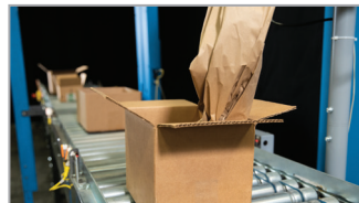
Sensor on tower measures box height as it moves through to determine correct amount of paper
