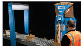
Void-fill material precisely dispensed into box with minimal assistance needed for packing
