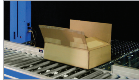
Rejecter technology automatically ejects out-of-queue boxes
